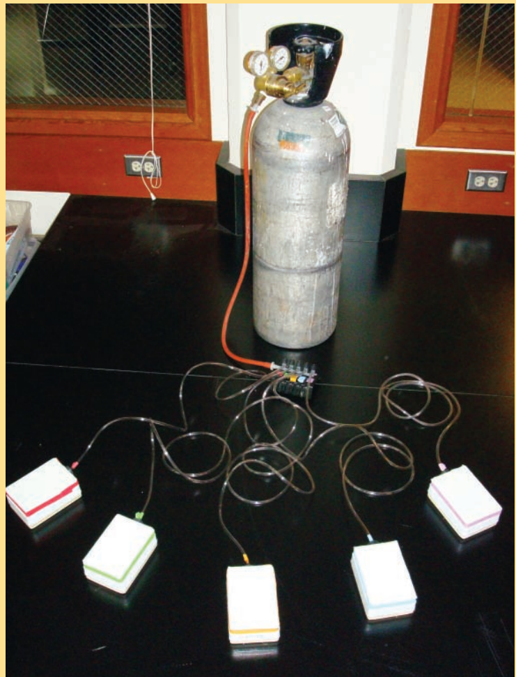
Figure 1. Photo of completed apparatus used to anesthetize Drosophila . The tank of carbon dioxide has been connected to a color coded five-gang aquarium valve that feeds five anesthetizing stages with aquarium tubing.
