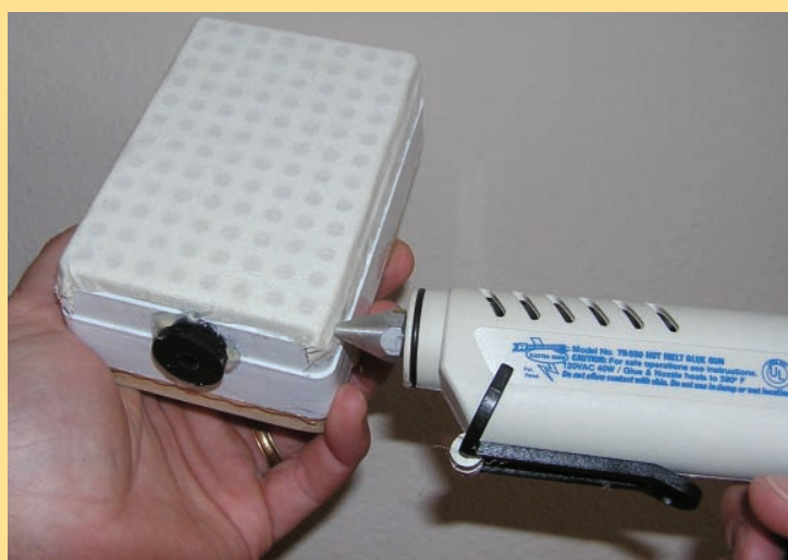
Figure 5. White felt or similarly porous fabric is placed over the top of the pipet tip box and secured around the edges with hot glue.
