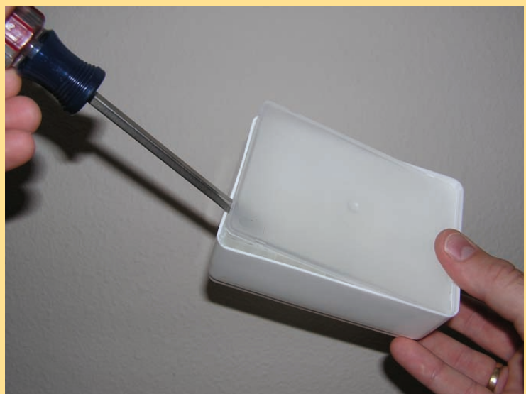
Figure 2. The base of the pipet tip holder is removed with a flat-head screwdriver.
