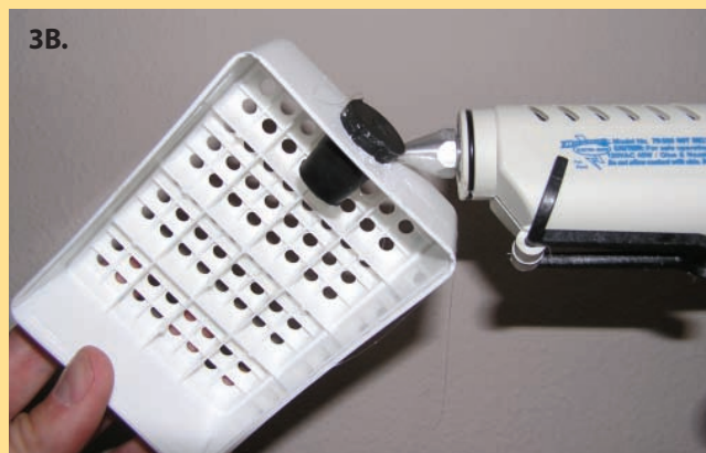
Figure 3A. A \frac{3}{4} " hole is drilled in the side of the pipet tip holder. 3B. The rubber stopper is inserted and secured with hot glue.
