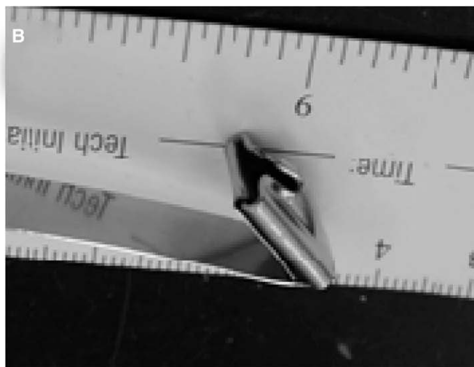
Fig. A2. Attaching the dendrometer band collar. (A) Slip a collar on the short section with the “tab” end of the collar away from the bend. (B) Fold the protruding short end of band under the collar and crimp the folds to secure the collar.
