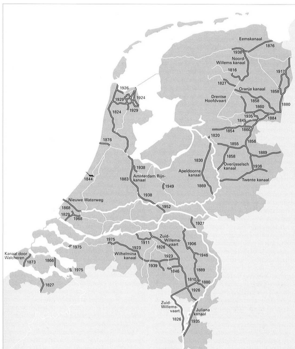
Figure 6. System of shipping routes developed by digging of channels in the nineteenth and twentieth century (van de Ven, 1993).
