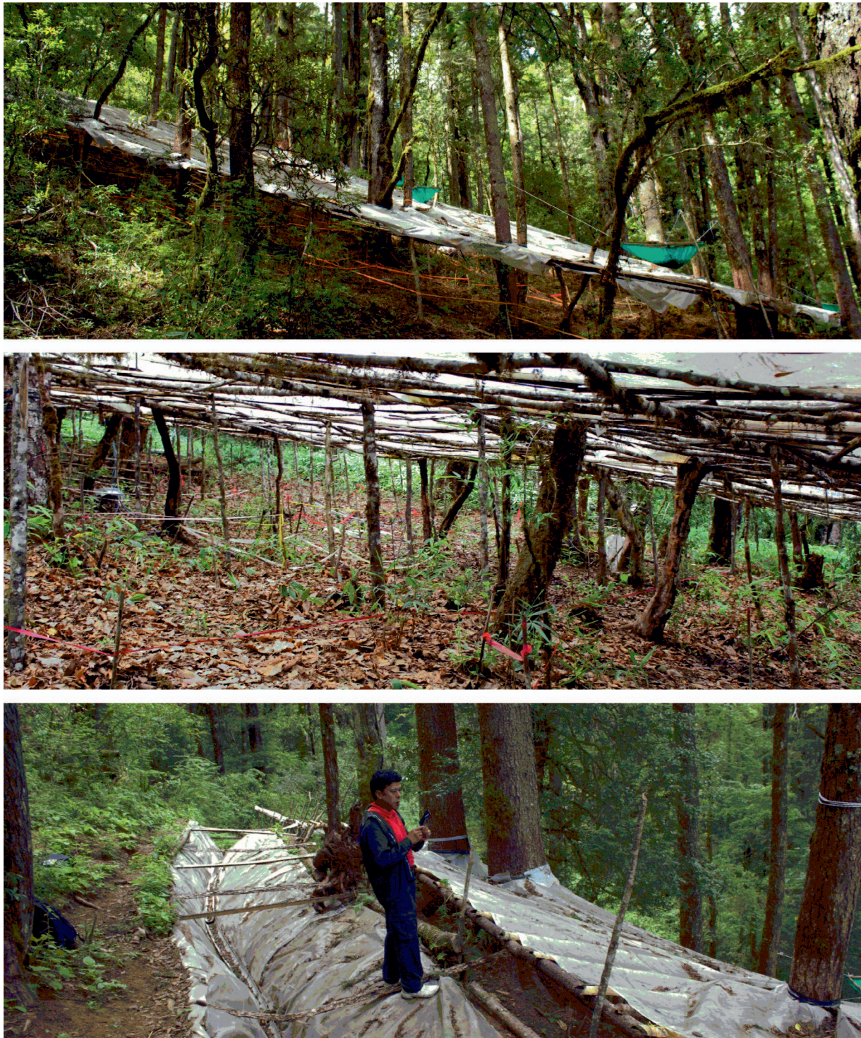
FIGURE 5 Experimental manipulation of precipitation using temporary plastic roofs (top) resting on 1–1.5 m bamboo poles (middle). Upslope of the roofed plot, a trench (bottom) was dug to prevent interflow of water.
